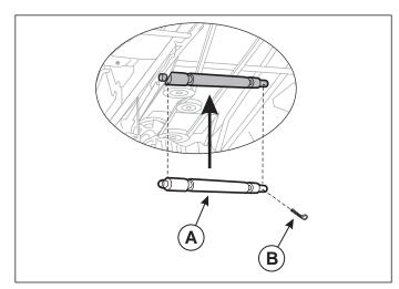
Figure 7. Hitch Support Shaft A. Hitch Support Shaft B. Cotter pin
